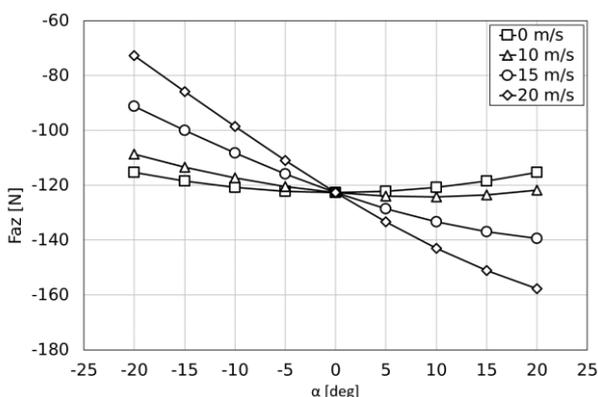
Figure 8. Theoretical model of  $F_{az}$  force for various wind velocities.
