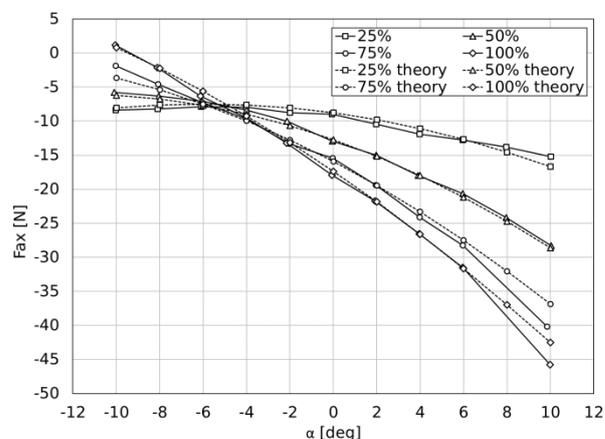
Figure 6. Comparison of experimental and theoretical data – Fax force.
