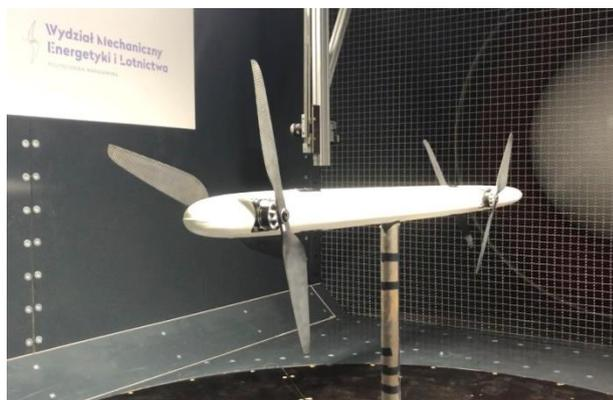
Figure 4. Tail-boom in the Wind Tunnel
