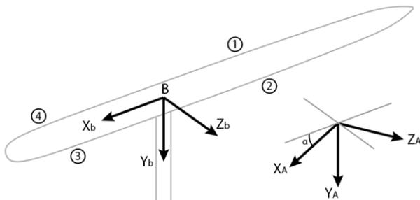
Figure 2. Tail-boom and aerodynamic coordinate system (compare with Fig. 4)
