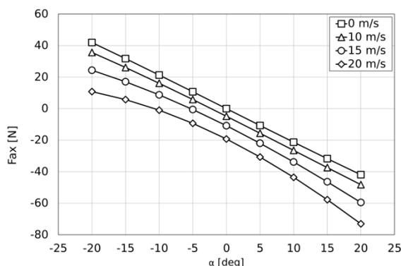
Figure 7. Theoretical model of  $F_{ax}$  force for various wind velocities.
